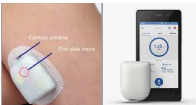
figure 6. Omnipod insulin pump by Insulet. Omnipod is the only tubeless patch insulin pump currently approved by the FDA in the U.S.
